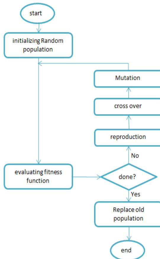
**Fig 2.** Genetic algorithm flowchart
